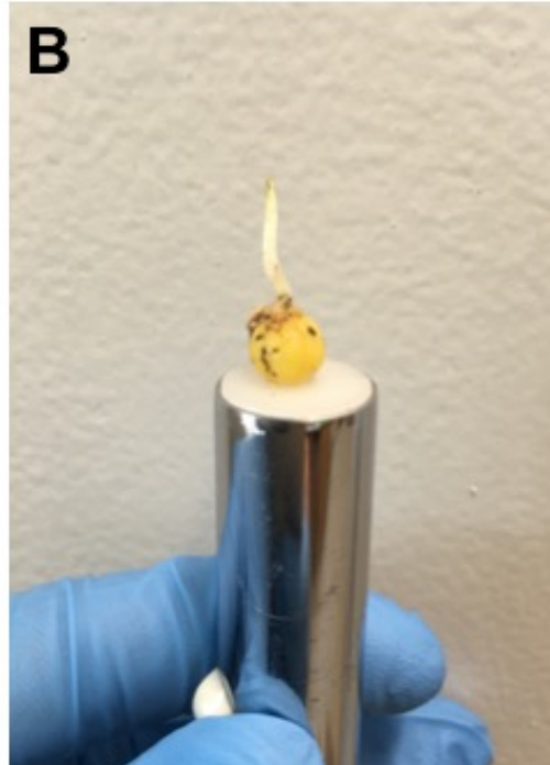
Figure 1. Preparation of plant specimen sectioning using the Compresstome™ slicer. (A) Newly germinated sweet pea specimen consisting of sprout stem, root, and seed pod. (B) Pea specimen is glued to the Compresstome™ specimen tube in an upright position ready for sectioning.
